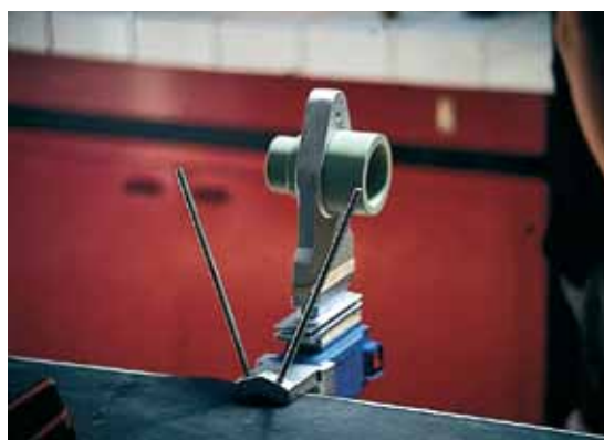
Photo 1: Appliance for manual joining of pipes and fittings by socket welding
